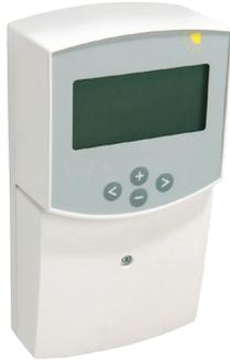
Electronic control unit for solar thermal systems with up to 2 solar panels with backlit LCD display. 8 different display configurations. Easy to use, with 4 interface pushbuttons. 4 Pt1000 sensors (ST Series-art. PPLELE00060) for solar collector, tank and auxiliary included as standard. The control unit is also set up to control 5 different control points (2 solar collectors, 2 tanks, 1 extra). It has:
